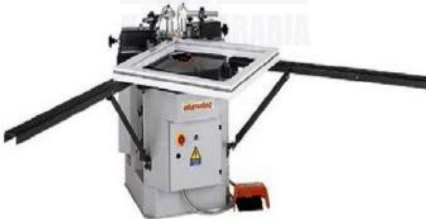
This machine is used for crimping of large dimensioned profiles to the highest quality standards. Easy adjustment and operation, short changeover times due to special blade changing system, special support head allows crimping of frames with in an inside dimension from 150mm.
