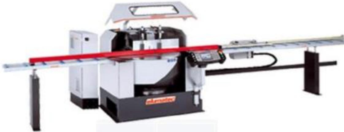
This machine also follows the principle of cutting from underneath. The patented saw arm suspension creates a cutting pressure towards the back fence which provides safe clamping of the workpiece. There is also free access for loading and unloading of profiles and automatically opens the safety of Hood.
